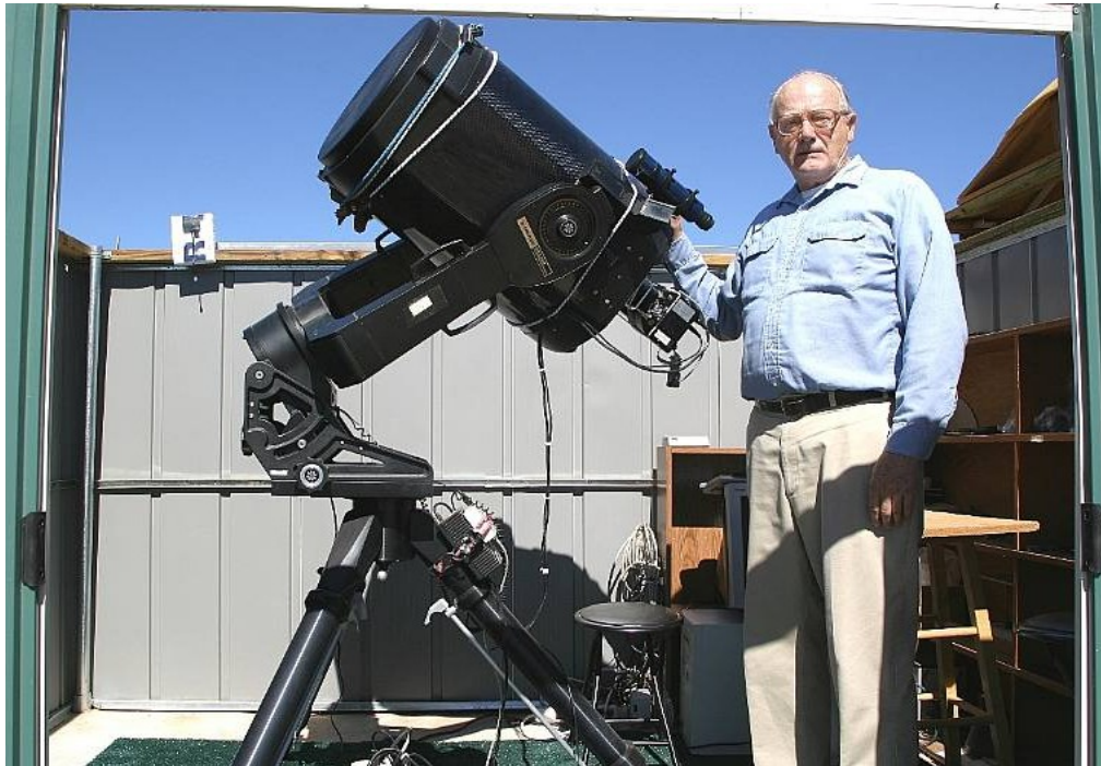
The author's favorite telescope, a Meade RCX400 14-inch on an equatorial wedge.
